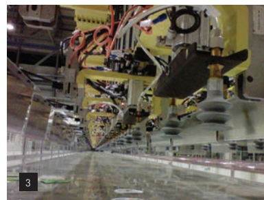
1 C series high-performance suction cup on robot line.
